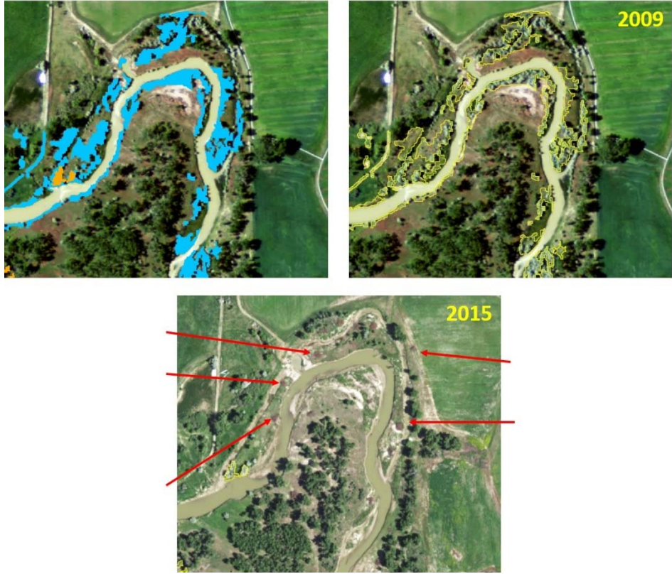
Figure 25. Example of active Russian olive removal along the Musselshell River. The upper pictures show patches that the model classifies as Russian olive in 2009 but not in 2015; in the bottom picture, red arrows point to scars resulting from recent Russian olive removal.
